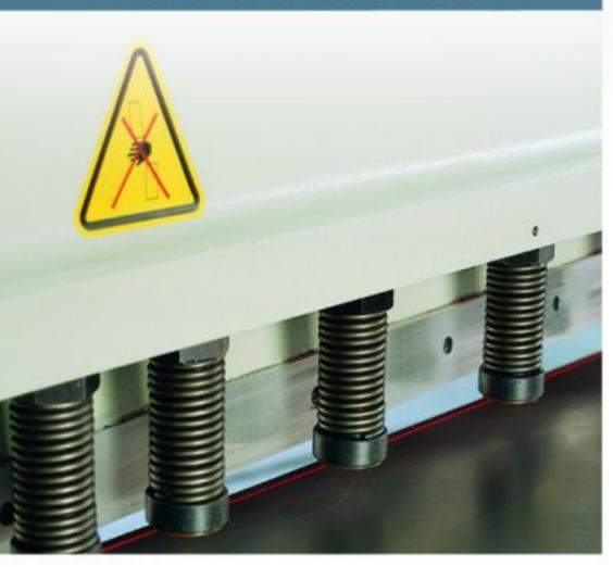
With the help of laser cutting line, angled or drawn line cuttings could be done easily and controllable. (Optional)
